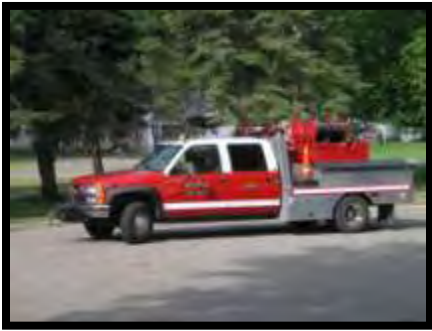
1997 Chevrolet Grass Rig 200 Gallon Tank 300 GPM 40 Calls
